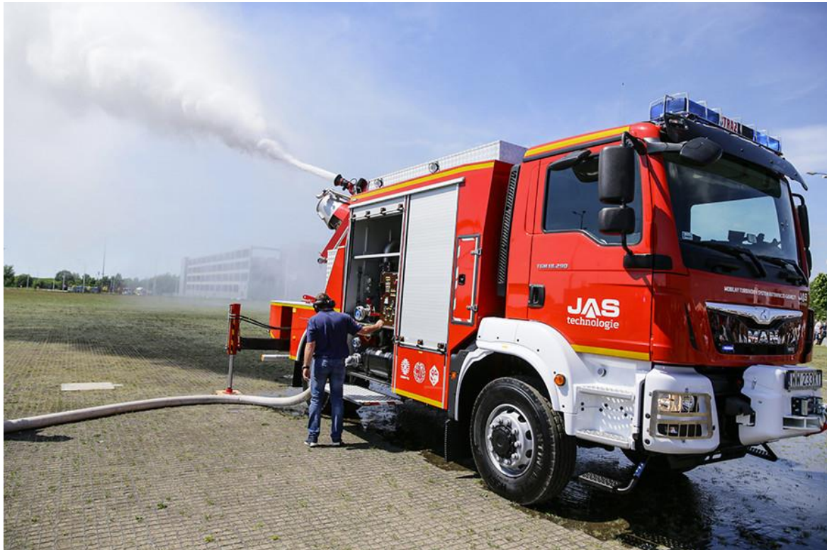
Fig. 2. Mobile turbine rescue and firefighting system Source: JAS Technologie
