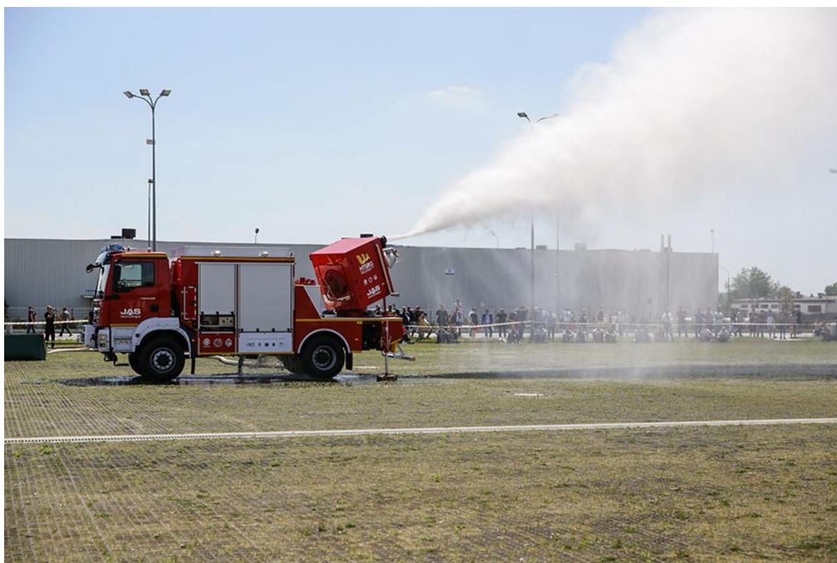
Fig. 1. Mobile turbine rescue and firefighting system
